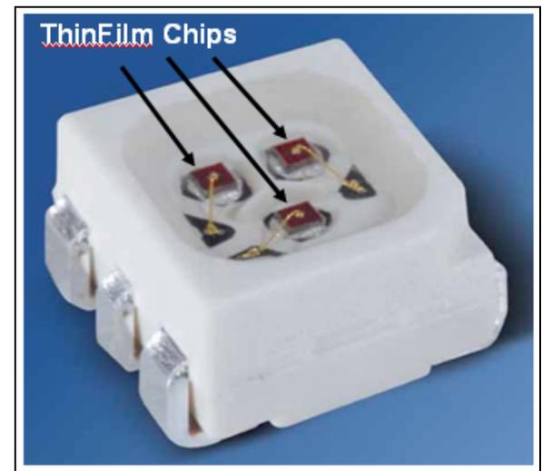
**Figure 4: 6-lead Multi TOPLED<sup>®</sup> with Thinfilm Chips and no ESD protection diode, due to space restrictions**
