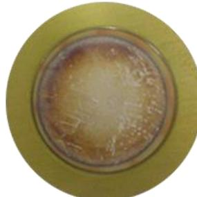
The electrode has turned black due to sulfidation.
